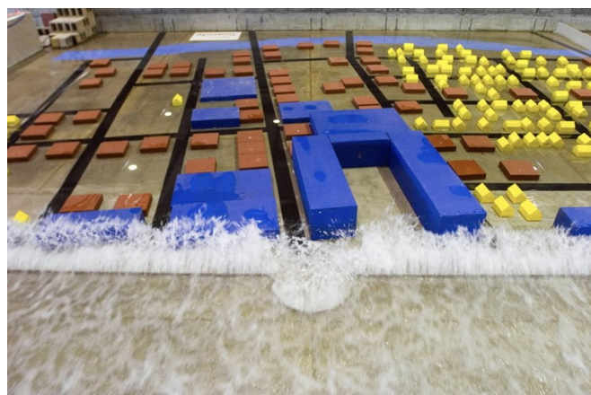
Town model of tsunami inundation performed at OSU's OH Hinsdale Wave Research Laboratory. Source: http://www.oregonlive.com/politics/index.ssf/2013/03/scientists_warn_oregon_legisla.html
